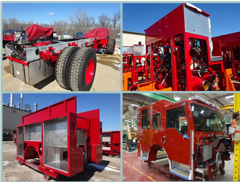
Clockwise from top left: frame and drive train; pump house; cab; fire body
