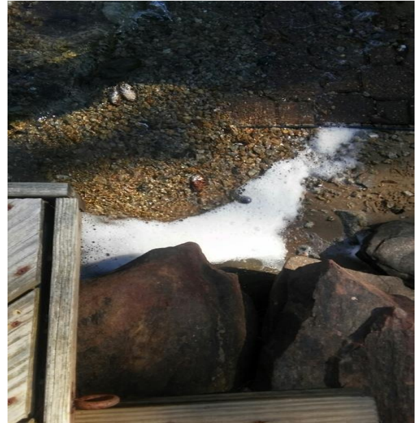
Soapy suds noted immediately below and adjacent to CAN-0317-OF, indicating greywater source.
