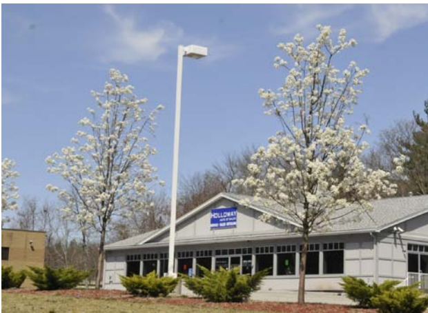
This light fixture has been coordinated with the planting plan to avoid problems as the trees mature. A slightly raised base protects the pole from plow damage.
