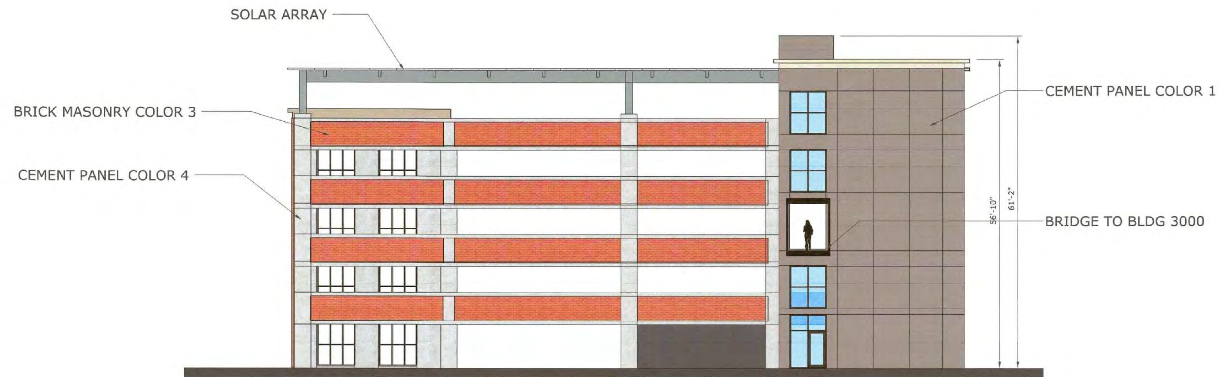
SOUTH ELEVATION BUILDING 3000 - PARKING GARAGE
