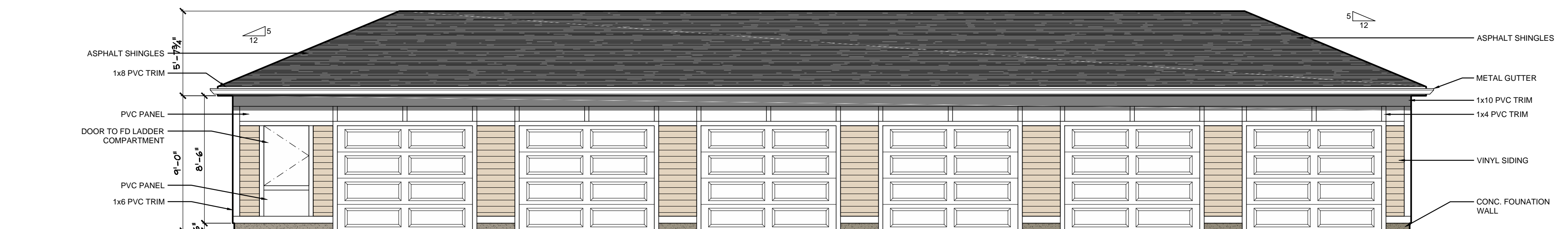
3 GARAGE BUILDING #3 - SOUTHEAST ELEVATION SCALE: 1/4" = 1'-0"
