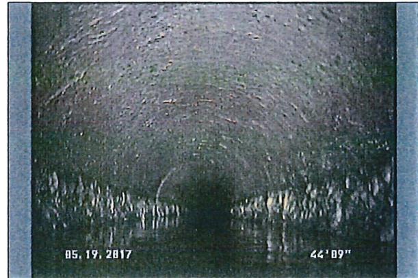
Photo: 1503 - 1504__19052017030913_A.JPG 44.75FT, Water Level, Sag in pipe, 40 %of cross sectional area
