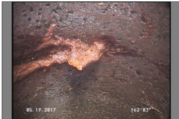
Photo: 116_13A, MPEG #: 050517_1, 00:07:15 162.25FT, Deposits Attached Encrustation, 5 % of cross sectional area, from 10 to 12 o'clock, within 8 inches of joint: NO
