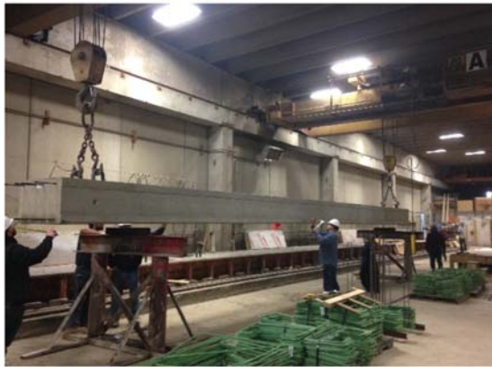
Removing one of the Completed Deck Beams from the Forms – Concrete Plant in Middlebury, VT
