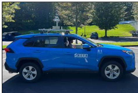
Figure 3: Image of BETA's hybrid vehicle equipped with lidar scanner
